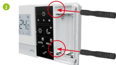
Use a screwdriver to push the plastic tabs in as shown in the figure until you feel resistance, and tilt the front part of the housing.
