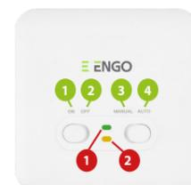
The status of the receiver is indicated by two LEDs. These are LEDs with the following colors:
