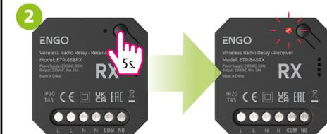
On the receiver(s) (RX), enter pairing mode by holding down the button for 5sec. The red LED will flash (pairing mode active).
