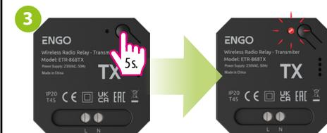
Then activate pairing mode on the transmitter (TX) by holding down the button for 5 sec. The red LED will flash (pairing mode active).
