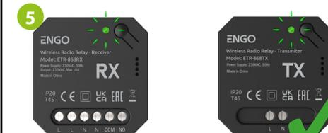
When the transmitter exits the pairing mode, it sends a signal to the receiver. LED diodes on both devices are green now. The devices are ready for work.
